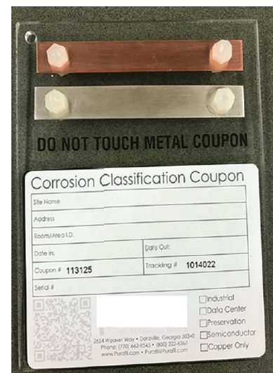
FIGURE 2 Example of copper and silver corrosion coupons.
